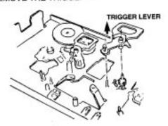
10. REMOVE CAM (A). TURN THE SCREW CLOCKWISE
