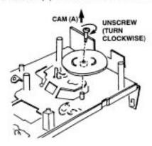
INSTALL THE NEW CAM (A). APPLY GL-701 GREASE ON THE SPOTS INDICATED. TURN SCREW COUNTER-CLOCKWISE
