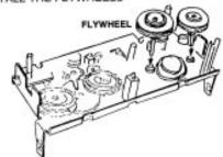
16. RE-INSTALL THE CAPSTAN MOTOR ASSEMBLY CAPSTAN MOTOR ASSEMBLY
