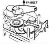
REMOVE THE CAPSTAN BELTS (A) AND (B), AND TENTATIVELY HOOK THEM ON TO THE MOTOR HOLDER
